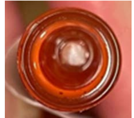
Figure 2. A tamper-evident cap tip broke off and remained in the syringe tip, preventing a nurse from administering the medication from the oral syringe.
